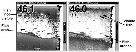
Sonar chart in regular grayscale mode (left) and FishReveal mode (right). Notice how shallow fish formerly hidden in the surface clutter become visible in FishReveal mode.
